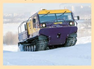
It is purposed for delivery of rotational shifts of workers, geological survey groups, trouble crews and for other transportation needs in off-road conditions at ambient air temperature from -40°C up to +40°C.
