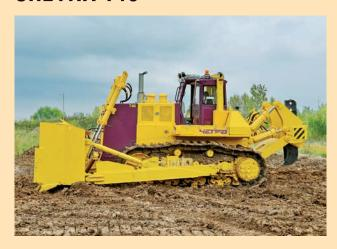
CHETRA T40 is the most powerful serial Russian bulldozer made for gold and coal mining industry.
