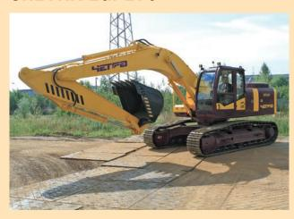
This shovel excavator is a multi-purpose earth-moving machine, designed for excavation of pits, trenches, open mines in soils of the 1-4 categories, loading and unloading of bulk materials, broken hard rock and frozen soils with maximum lump size 400 mm, as well as for other industrial, municipal, agricultural, transport and land reclamation applications.
