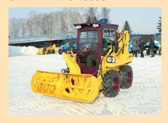
MKSM 800C mini-loader with carrying capacity 800 kg is equipped with diesel engines by Cummins (South Korea) with liquid cooling system. This loader features lower noise level.
