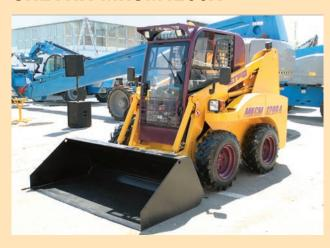
MKSM1200A mini-loader with carrying capacity 1 200 kg is developed with application of state-of-the-art technologies, innovative solutions and original cab design. This loader is purposed for road construction and industrial construction, municipal operations.
