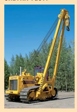
This pipelayer is the best choice for those who need an advance machine with maximum lifting capacity. It can be used for laying pipes of diameter from 900 to 1 420 mm.
