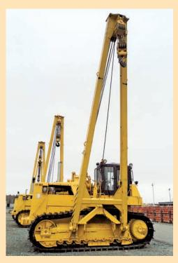
A simple and reliable machine for heavy duty pipelaying operations. It can be used for construction of main gas pipelines with pipe diameter from 900 to 1 420 mm.
