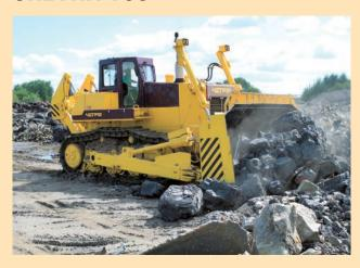
This is a powerful bulldozer for heavyduty earthmoving and stripping operations including excavation of frozen and rocky soils.
