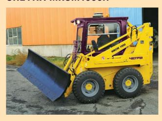
**MKSM1000H** mini-loader with carrying capacity 1 000 kg is purposed for operations in road construction and industrial construction, municipal operations.
