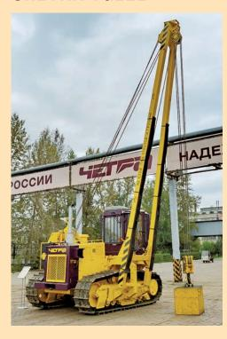
This is a light pipelayer for laying oil pipelines and water pipelines. It can be used for operations with pipes of diameter from 400 to 600 mm.
