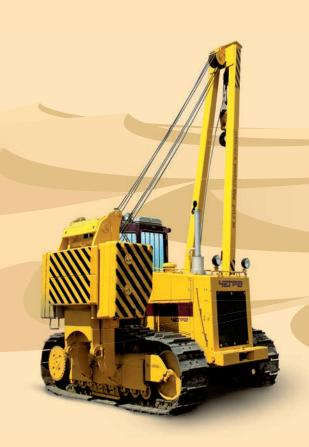
Concern Tractor Plants offers a wide range of pipelayers with lifting capacity from 26 ton up to 104 ton for handling operations in civil and petroleum construction. The pipelayers are designed for laying steel pipes with diameter from 8" to 56".
