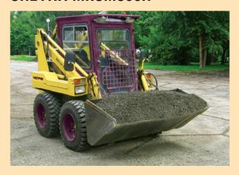
**MKSM800H** mini-loader with carrying capacity 800 kg has showed itself to good advantage in such applications where, due to narrowness or due to economic reasons, it is impossible or ineffective to use standard large scale machines.
