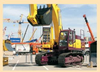
This is the most powerful CHETRA excavator designed for industrial and road construction applications, as well as for subsidiary works in open mines.
