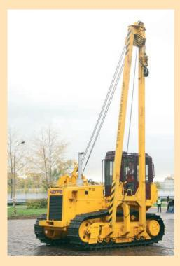
A most popular CHETRA pipelayer for laying pipes into trenches, escorting pipe-swabbing & isolation machines and handling of unit loads.
