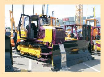
This is a compact bulldozer which, due to its size, can be transported in a truck body without obtaining a special permit.
