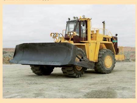
It is purposed for road-construction operations, work on coal storage facilities, levelling of tailings surfaces, areas for excavators and drill rigs and as a hauler when transporting heavy cargos or a pusher for railroad cars. It features high maneuverability and productivity. It is ideal for minor auxiliary work in dispersed areas.
