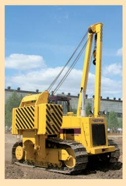
This is a medium range pipelayer used for construction of pipelines of diameter from 600 to 1000 mm.
